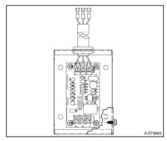
Figure 6-30 Single-Relay Dry Contact Kit, Typical
